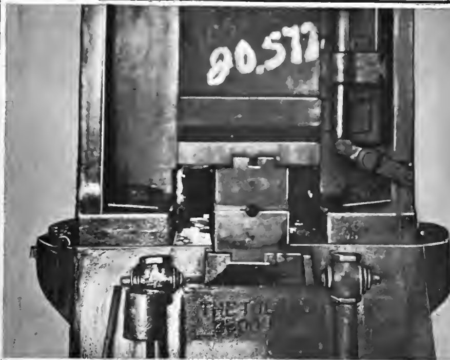
D—A 2,500-Pound Toledo Hammer Working on Drop-forged Crankshafts of 40 Carbon Steel, This Being One of a Considerable Battery of Hammers in the New Overland Drop-forge Plant
